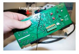
5. Pull the logic board towards the side of the opener to disengage the black retaining hooks. Finish by removing the logic board. To install the logic board repeat all steps in reverse.
