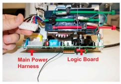
3. Remove the main power harness from the logic board. Gasp the main power harness between your fingers and pull up lightly until it disengages from the logic board.
