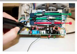
4. Remove the limit system wire assembly from the logic board. Gasp the limit system wire connection between your fingers and pull lightly until it disengages from the logic board. Remove the two retainings screw on the logic board using a Phillips screw driver.
