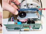
3. Remove the limit system assembly. First remove the limit wire from the logic board. Second push in the three tabs with your finger until you feel them disengage. Finish by pulling up gently on the limit system assembly to disengage.
