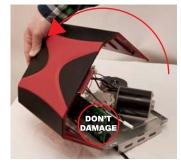
5. To remove the plastic motor cover grab the front of the plastic motor cover & swing up towards the back of the opener. <u>Take care</u> not to damage any of the buttons on the logic board. Once removed the opener should look like this ->
