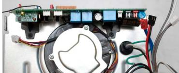
6. Remove all of the five wire connections (A-E) connected to the logic board. Connections A & B will pull directly off. Connections C, D, & E require you to press & release a clip located on the bottom of each connector. Once the clip is pressed, remove the connection.
