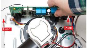
7. Using a Phillips screwdriver remove the two screws securing the logic board to the opener chassis. Disengage the logic board by pushing the logic board away from motor. Once disengaged pull straight up to remove. Repeat all seven steps, in reverse, to install the logic board.
